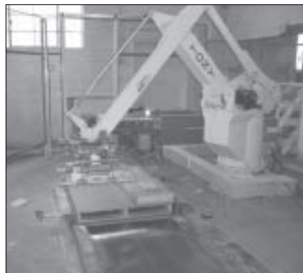
The Columbia/Okura robot in Big J Milling's Brigham, UT facility packs 10 flour bags per minute onto a pallet.
