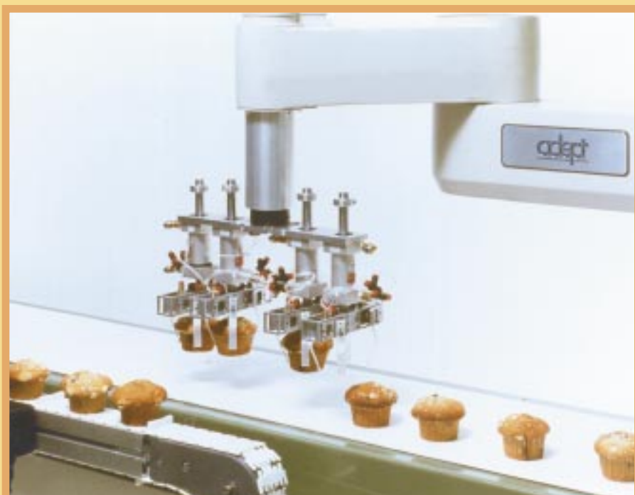
Robotic packaging systems are making inroads in the food industry, where rising labor costs and ergonomic issues are prompting companies to look at flexible automation.
