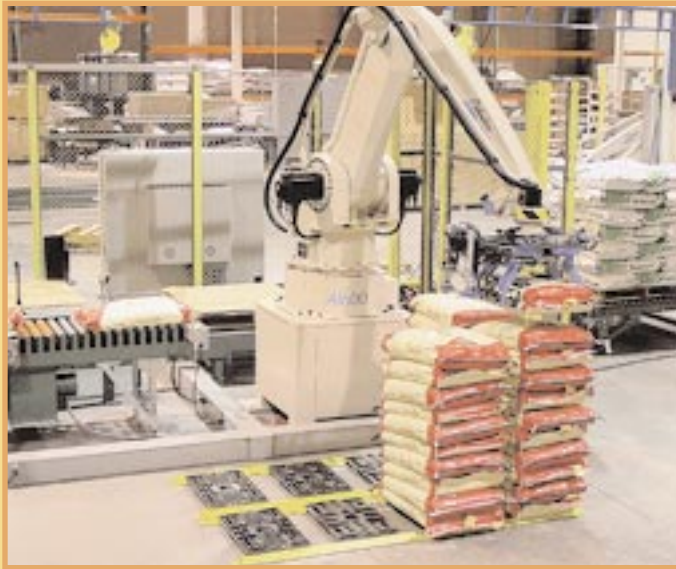
Robotic palletizing systems offer versatility not found in traditional palletizing unitizers. This Columbia/Okura palletizing robot can stack bags either on a standard pallet or on a single-stack pallet for individual orders.
