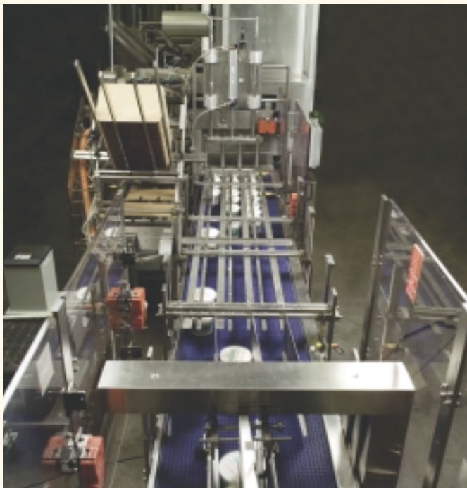
Delkor's new Servo Laner accommodates rapid changes for pack patterns and cup sizes.
