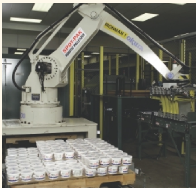
The new SPOT-PAK® Robotic Palletizer is designed to handle the full range of SPOT-PAK® packages.
